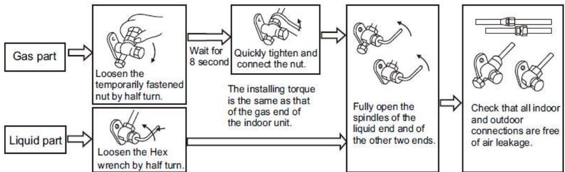
**★Vacuum Pumping Method (R410A refrigerant evacuation must use the vacuum pumping method)**
