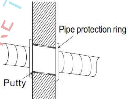
**Note: Usually, the wall hole is  $\Phi 60\text{mm}$ ~ $\Phi 80\text{mm}$ . Avoid pre-buried power wire and hard wall when making the hole.**
